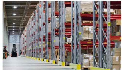
Even in a state-of-the-art warehousing operations the standard pallet racking system is still the most common form of pallet racking storage.
